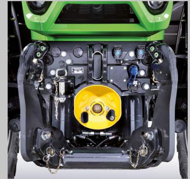
Integrated front linkage with unique short distance to the front axle. Less overhang. Superior tractor balance.
