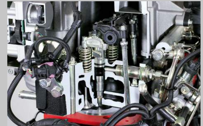
DCR technology. 2,000 bar injection pressure ensures maximum engine efficiency.
