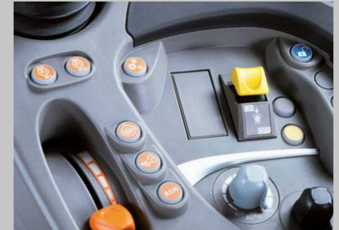
The PTO settings and activation are conveniently integrated into the armrest ...
