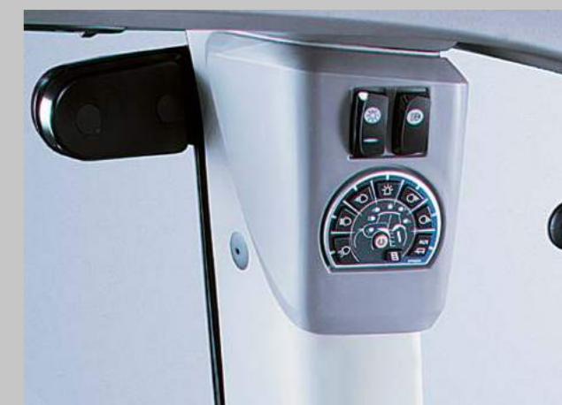
Driving lights, work lights and cab light combined in a single control panel.
