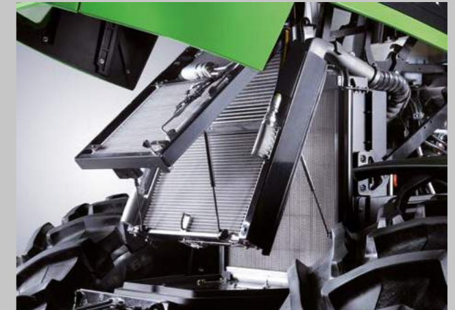
The radiator can be quickly unfolded and cleaned.
