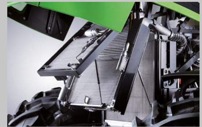
The compact cooling system enhances engine efficiency and is easy to maintain.
