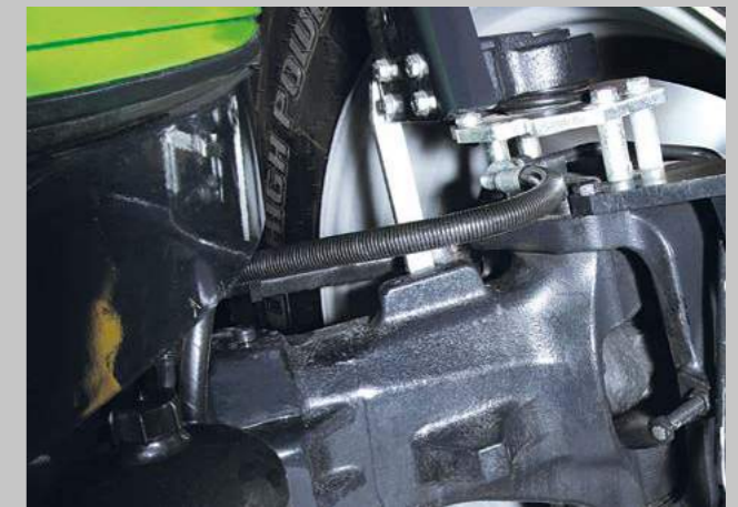
Front axis. Maximum spring effect and a steering angle of up to 50 degrees.
