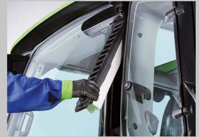
The cab air filter in the cab post can be easily accessed without tools.
