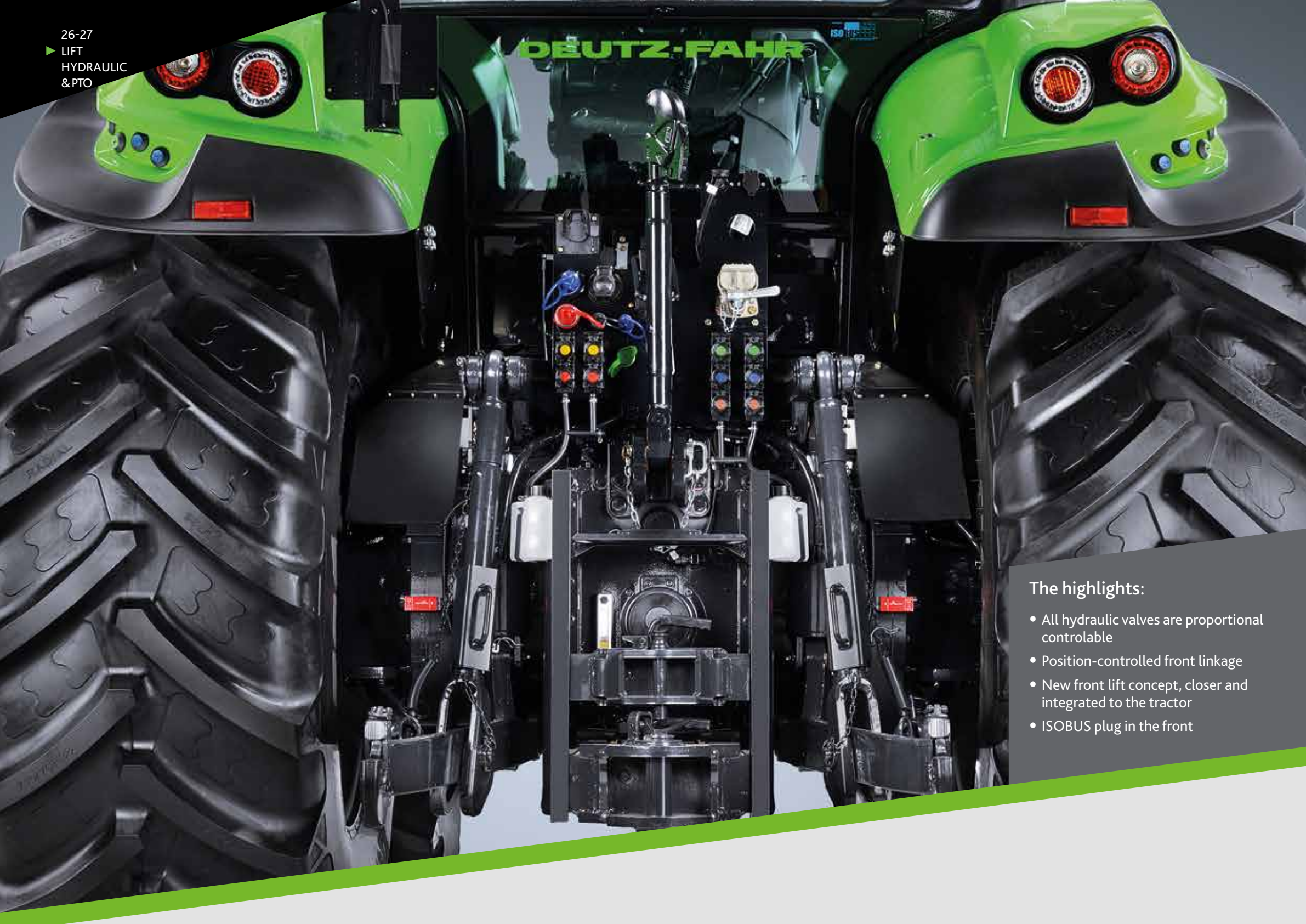
Up to 5 proportional spool valves in the rear and 2 in the front. Front lift closer and integrated to the tractor.
