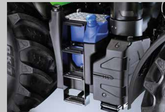
Less fuel and AdBlue consumption. 400 L diesel and 50 L AdBlue tank for long working sessions.
