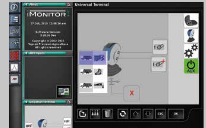
VT4 ready. Implement functions controlled by tractor own buttons.
