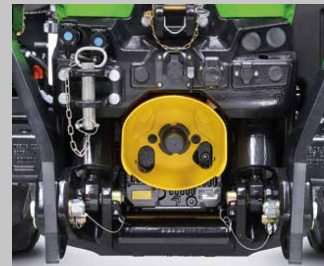
Up to 5 proportional spool valves in the rear and 2 in the front. Front lift closer and integrated to the tractor.
