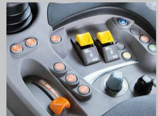
PTO controls (front/rear) and engagement handily integrated in the armrest...
