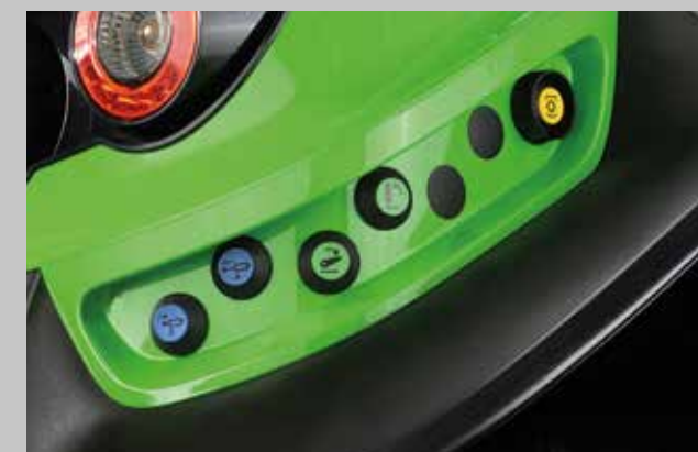
External control of hydraulics, rear lift and PTO from both sides.
