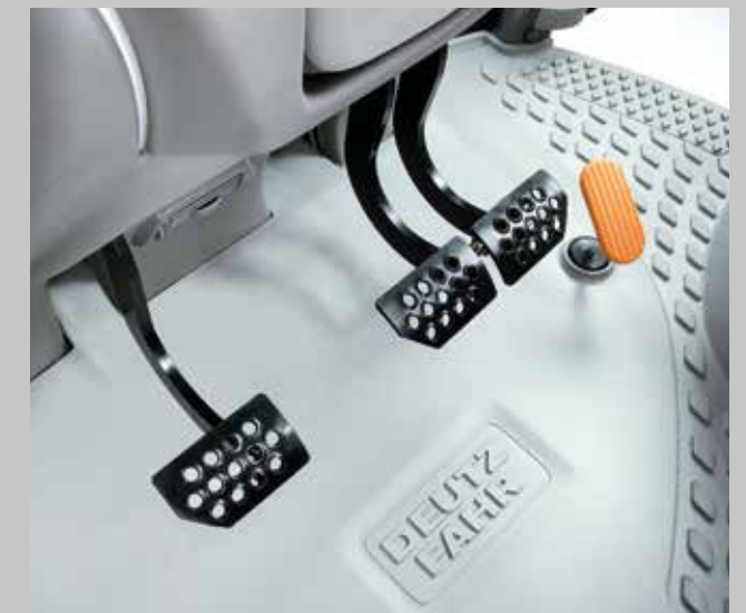
Booster brake system ensures high braking performance with low pedal force.
