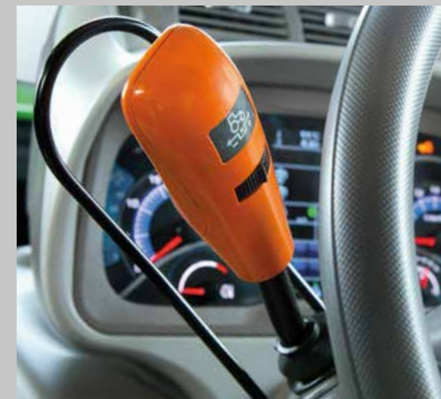
PowerShuttle with SenseShift, the 5 levels of reversing sensitivity can be easily adjusted.
