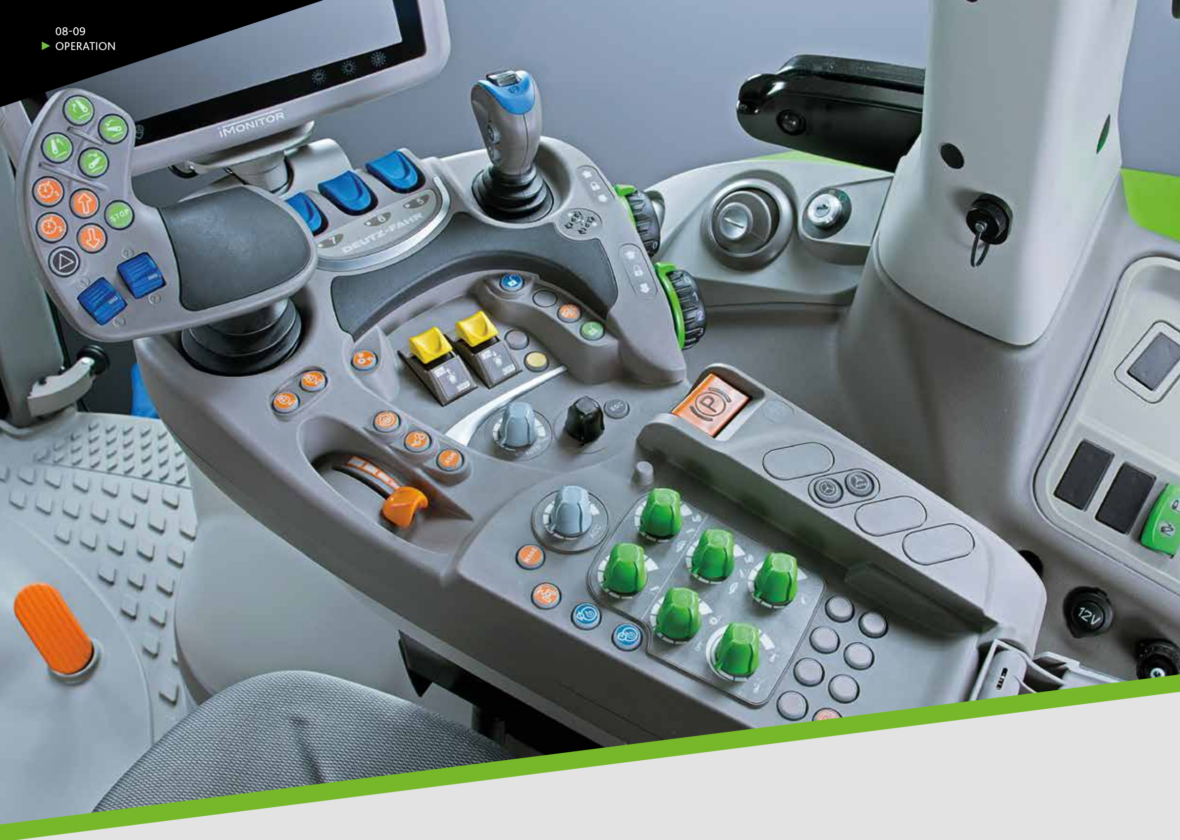
PTO controls (front/rear) and engagement handily integrated in the armrest...
