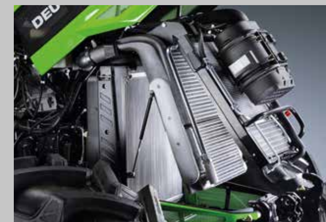
New designed cooling system. Fully openable for easy maintenance.
